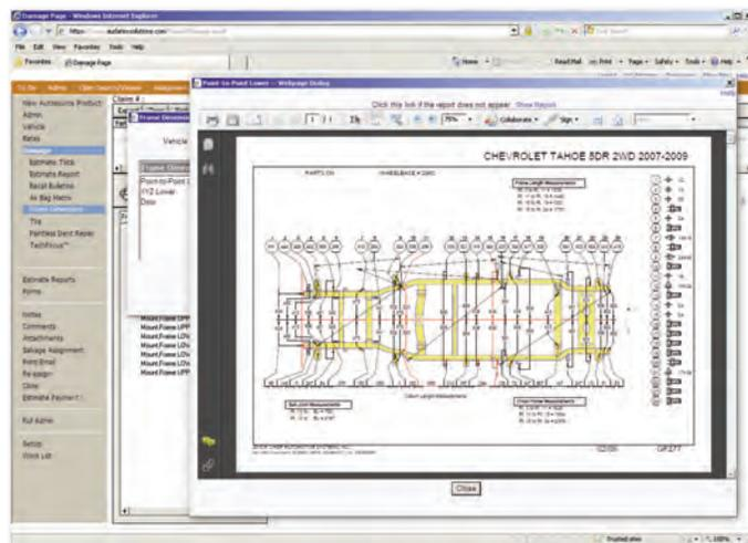
FRAME DIMENSIONS INCLUDES SPECIFICATIONS FOR POINT-TO-POINT, CENTERLINE AND DOOR OPENINGS
